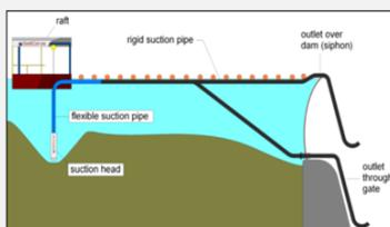
Figure 2. SediCon Dredge Section View. Image from SediCon
