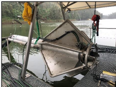
Suction head used to liberate lower gates in Necaxa, México
