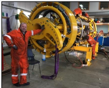
Tool for dredging inside piles, designed by SediCon
