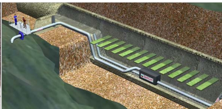
SediCon Sluicer in tunnel sand trap
